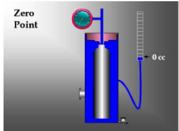
To identify any temperature related problem, load the cylinder into the test jacket, seal the head and log the expansion readings at 30 second intervals in a form similar to the one below: Example readings are shown.
