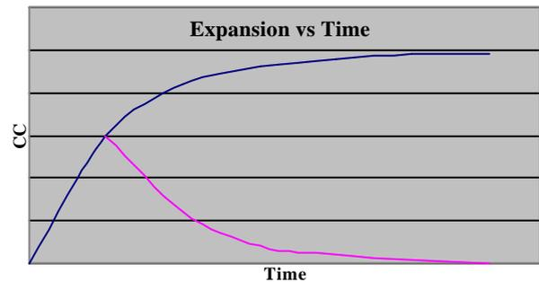
The graph shown the expansion gradually reaching a steady value. It can be plotted either as the expansion value itself (in which it tends to reach a stable value) or as the change from the last reading – this will tend towards zero. Values could be increasing or decreasing. A straight line or steady expansion change over time represents a leak – not at temperature effect!
